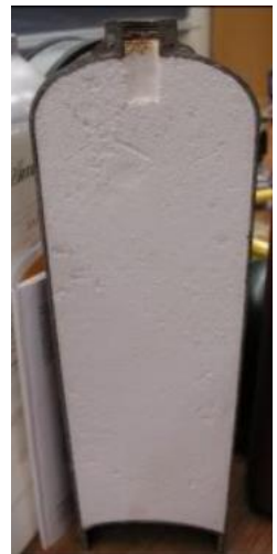
Here is a cross section of an acetylene cylinder. It shows the monolithic filler material and the open area near the valve that the gas separates itself out of the acetone or DMF that it is dissolved in when the cylinder is filled.
